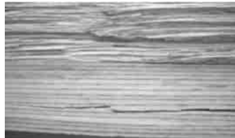
图 7 单板间撕裂破坏 Fig. 7 Fracture surface of tearing in the veneers
