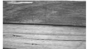
图 8 胶层剪切破坏 Fig. 8 Fracture surface of shearing in glue layers
